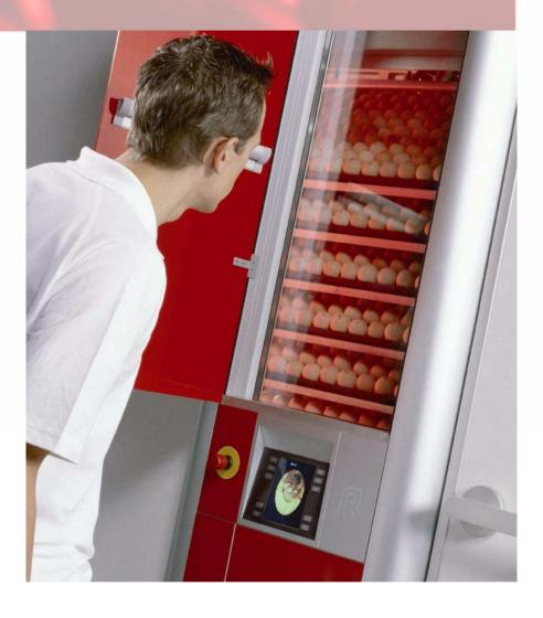
Homogenous temperature distribution is the single most important parameter for successfully incubating today's modern breeds, each of which has a unique temperature 'signature' for embryonic development. Even minor temperature fluctuations can have a major impact on uniformity and post hatch performance. With SmartSet™, the average difference in eggshell temperature is less than 0.5 °F.
