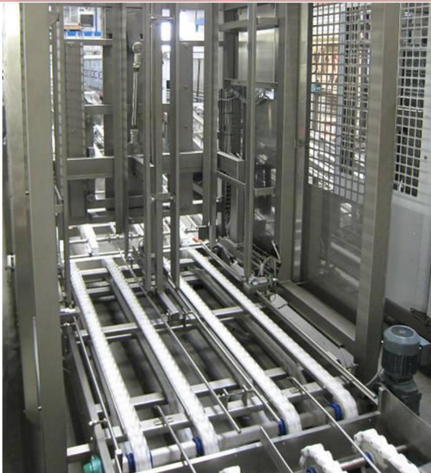
**Automatically supplies empty hatcher baskets and/or chick boxes from stacks to a washer or chick counter – or removes and stacks washed hatcher baskets and/or empty chick boxes.**
