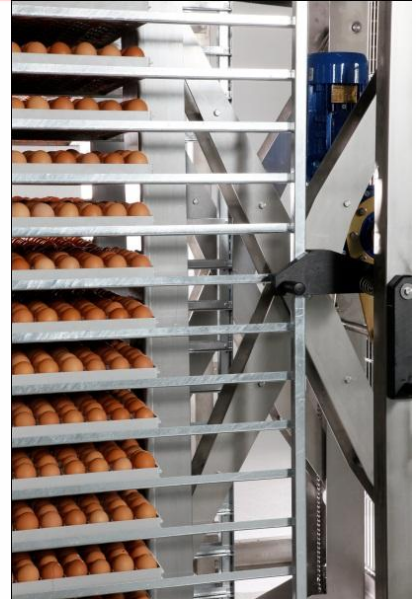
In a single, smooth movement, the pusher (right) moves all the setter trays onto the tray collector
