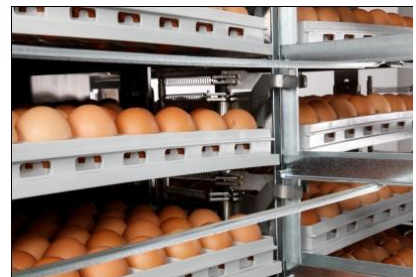
The tray collecting system automatically extends grabs, to lock the setter trolley into position
